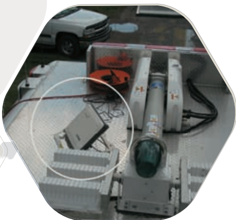
Compact BGAN satellite terminal (circled) on top of a Hazmat vehicle, connected to a laptop, during a biological incident in rural Kentucky. Photo courtesy of Mark Garland, Murray State University.
