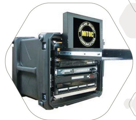
The Man-portable Interoperable Tactical Operations Center (MITOC) was developed based on commercial off-the-shelf technologies—including BGAN from Stratos. Photo courtesy of the University of Louisville's iTRC.
