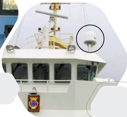
Thrane & Thrane SAILOR 500 FleetBroadband antenna (circled).
